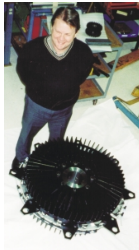
Dover Flexo application engineer, Walter Rothe, beside a 3000 series dual disc brake assembly. (Note the dual disc for a 60 series brake over Walter's left shoulder.)
