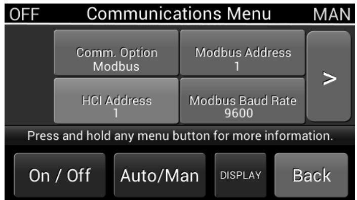
Figure 7 - SETUP MODBUS COMM
