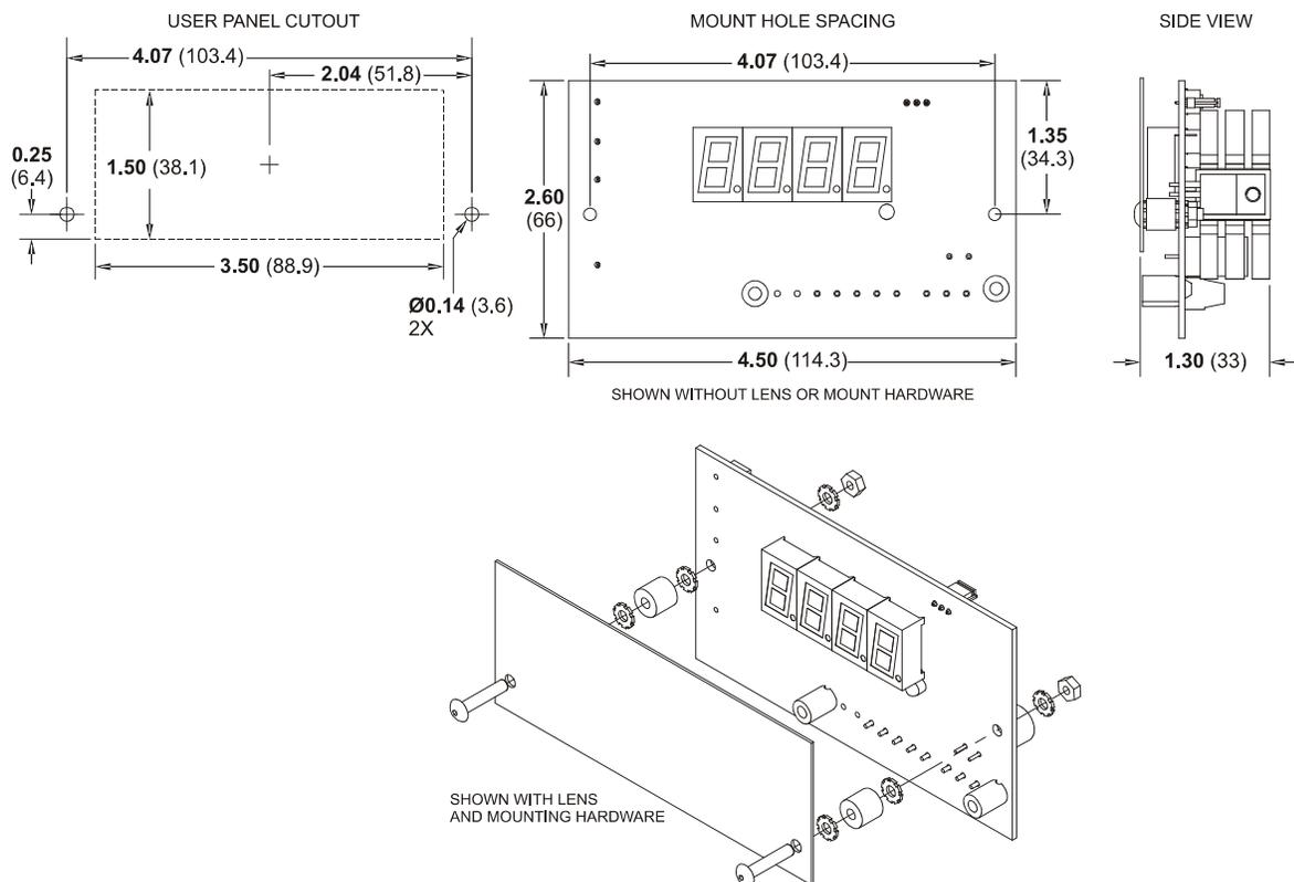
**Figure 1 - DIGITAL METER DIMENSIONS AND PANEL CUTOUT DIMENSIONS**
