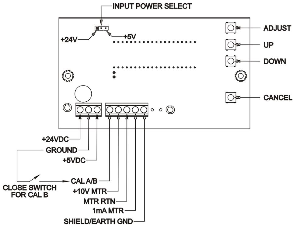
**Figure 2 - DIGITAL METER BOARD WITH CONNECTIONS AND ADJUSTMENTS**
