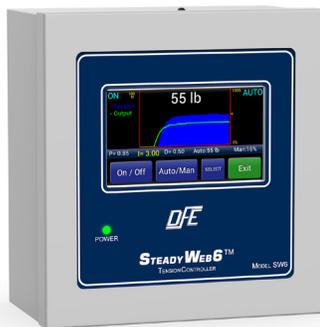
A closed-loop electronic control system can provide far greater accuracy and repeatability than a manual system. In a closed-loop control system, we replace the operator's judgment and intuition about how much to adjust a tensioning device's output with an electronic controller's control algorithm.
