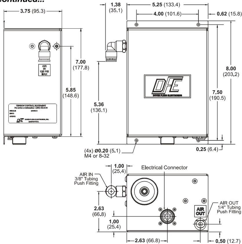
**Figure 5 - PNEUMATICS ENCLOSURE DIMENSIONS FOR VERSION P**
