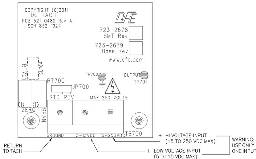
**Figure 32 - DC TACHOMETER CARD**
