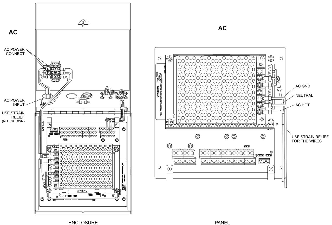
**Figure 11 – AC POWER ELECTRICAL CONNECTIONS**
