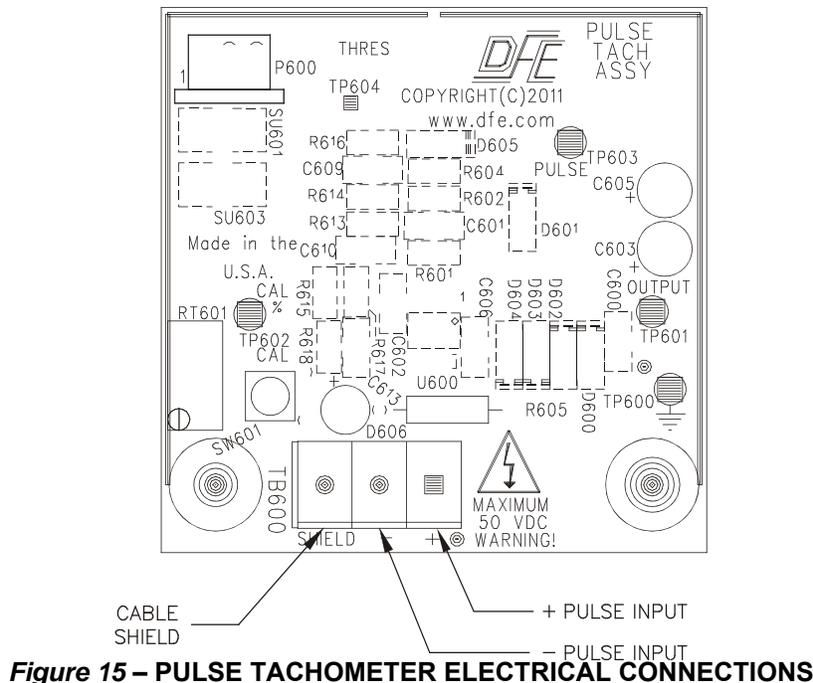
**Figure 15 – PULSE TACHOMETER ELECTRICAL CONNECTIONS**
