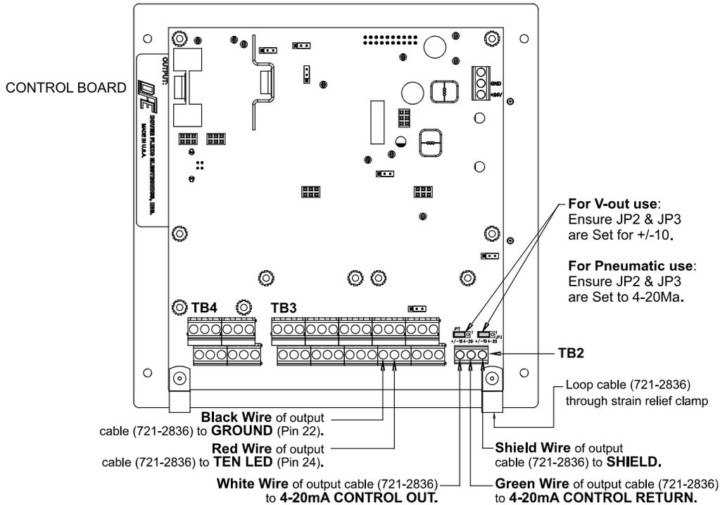
Figure 18 – EXTERNAL OUTPUT MODULE CABLE CONNECTIONS
