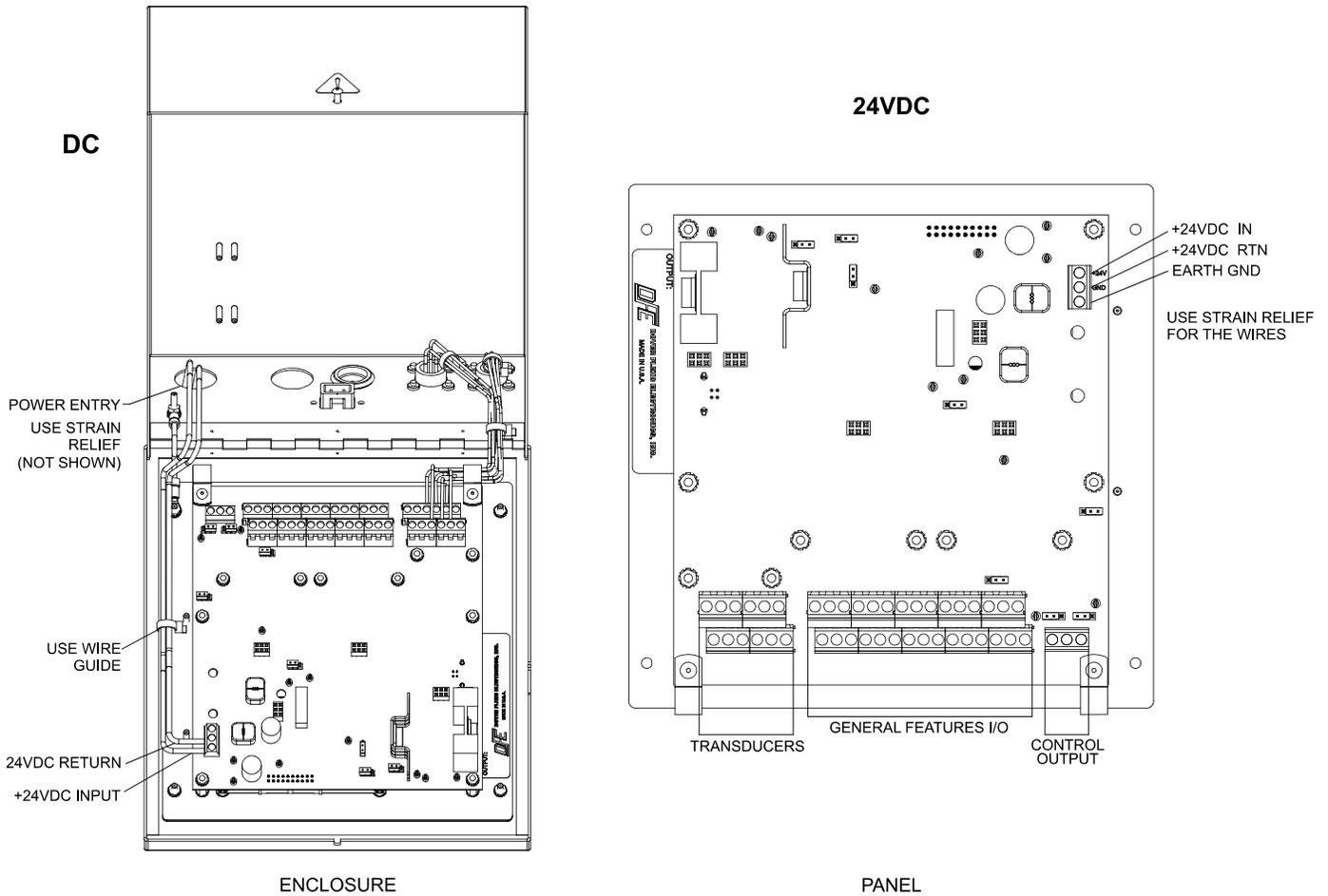
**Figure 10 – 24VDC POWER ELECTRICAL CONNECTIONS**
