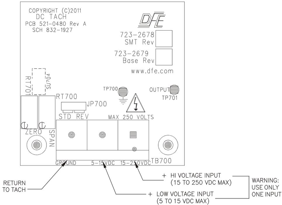
**Figure 16 – DC TACHOMETER ELECTRICAL CONNECTIONS**
