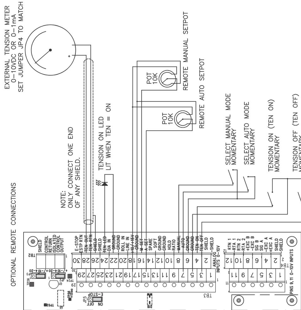
Figure 50 - CONTROL BOARD TRANSDUCER ELECTRICAL CONNECTIONS AND REMOTE OPTION
