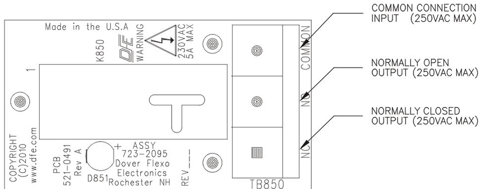
**Figure 17 – RELAY ELECTRICAL CONNECTIONS**
