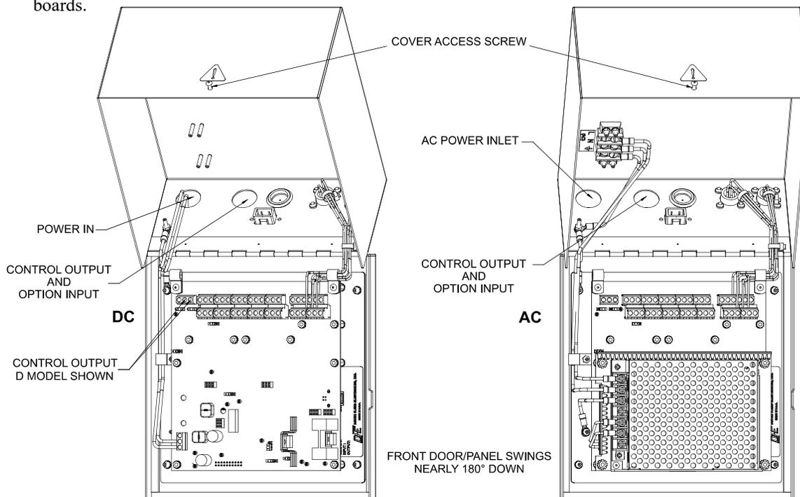
**Figure 7 – ENCLOSURE VERSION SERVICE ACCESS**
