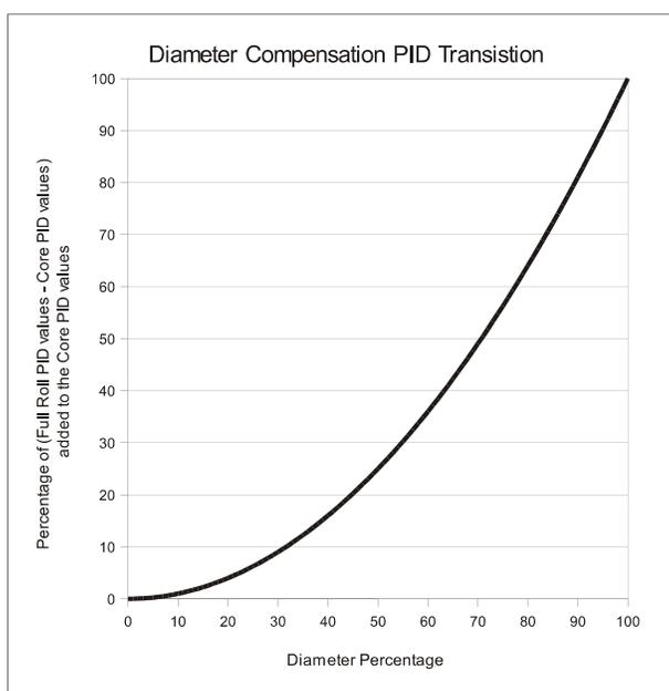
Figure 39 – DIAMETER COMPENSATION PID TRANSITION
