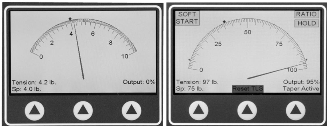
**Figure 23 – ANALOG METER DISPLAYS**
