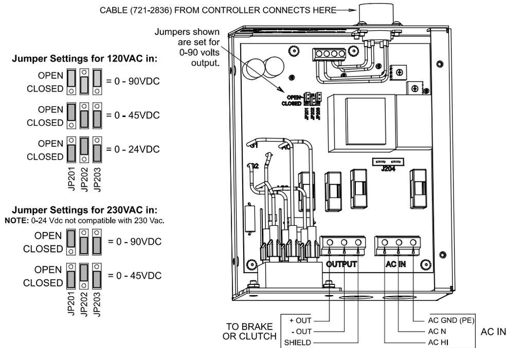
Figure 19 – HIGH VOLTAGE OUTPUT MODULE ELECTRICAL CONNECTIONS
