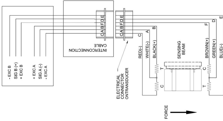
Figure 52 - MODELS RFA, LT, & VNW TRANSDUCER WIRING
