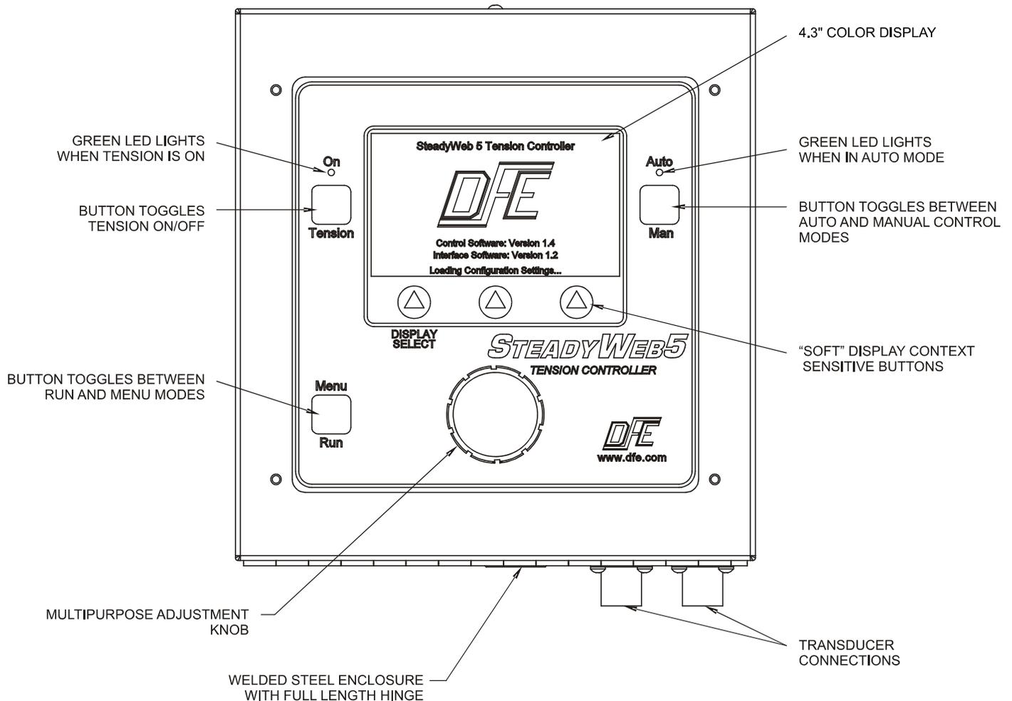
Figure 1 - FRONT VIEW OF STEADYWEB™5
