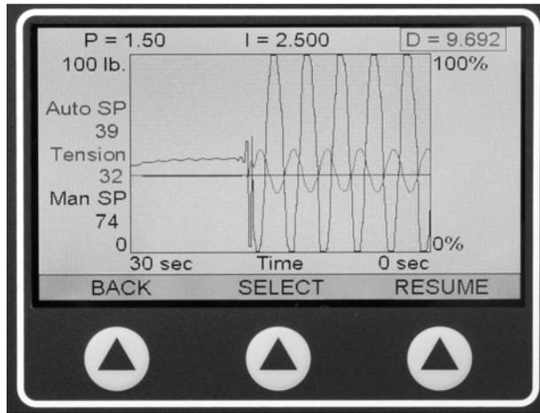
**Figure 37 – TUNING SCREEN SHOWING DERIVATIVE NOISE**
