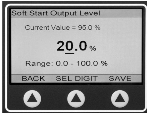
**Figure 27 - SOFT START OUTPUT LEVEL ADJUSTMENT DISPLAY**
