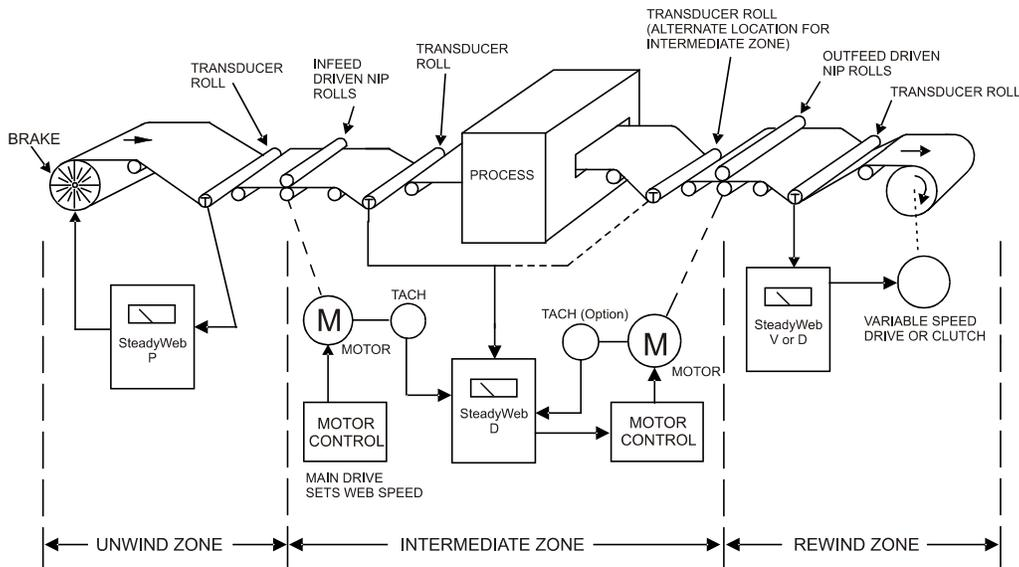
**Figure 2 - EXAMPLES OF TENSION ZONES**
