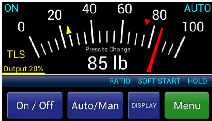
Figure 19 - TLS SETPOINT SHOWN
