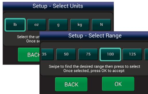
After confirming or selecting new tension units, the controller will similarly guide you through selection of the tension range, the source of the tension signal, calibration weight percentage and transducer type to be used. The tension range should be set at, or just above your expected upper web tension limit.
