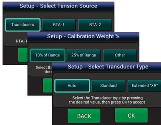
**5** With no other loads on the transducer roll, **ZERO** the transducers, hang a calibration weight of known value with an inelastic rope, strap or cable, and **CALIBRATE** the transducer signal, exactly as instructed in Section 4.1.1 of **The Manual**. The calibration weight should weigh at least 10% of your maximum expected web tension.
