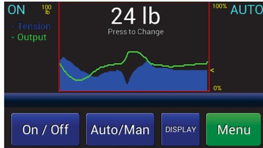
**10** When in tension display screens, you may bring up velocity-sensitive “+” and “-” adjustment buttons by touching the tension display. These buttons, for adjusting the Auto Setpoint or Manual Output will time out a few seconds after discontinued use.
