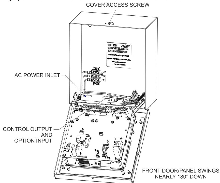
**Figure 7 – ENCLOSURE VERSION SERVICE ACCESS**
