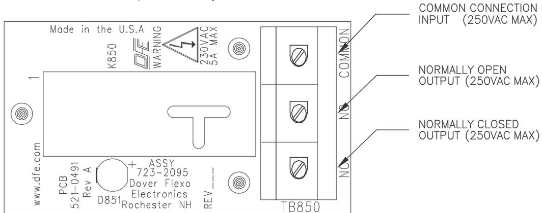
**Figure 17 – RELAY ELECTRICAL CONNECTIONS**
