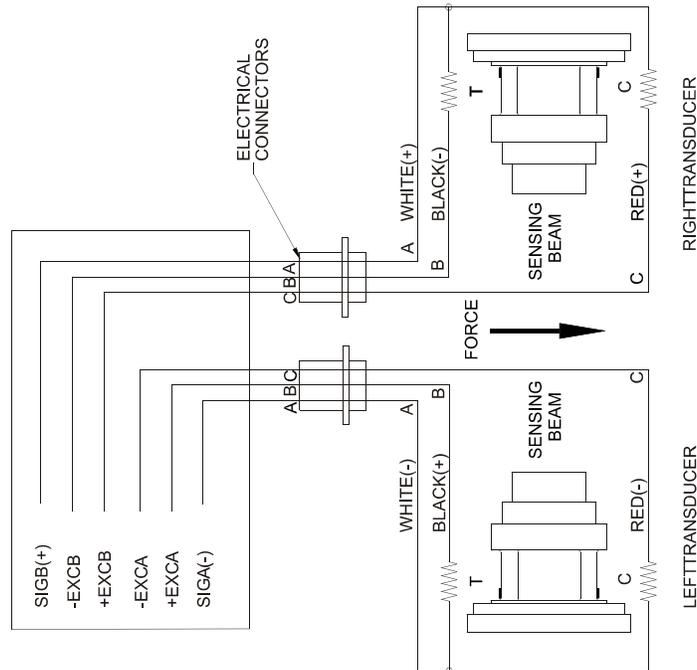
Figure 48 - MODELS C, RS, F, TR, & NW TRANSDUCER WIRING
