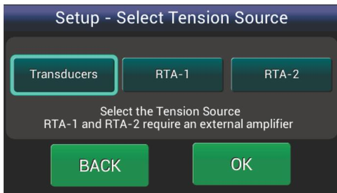
Figure 26 - SELECTION OF TENSION SOURCE
