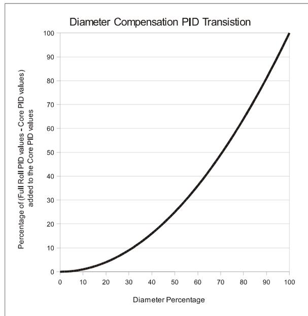
**Figure 43 – DIAMETER COMPENSATION PID TRANSITION**
