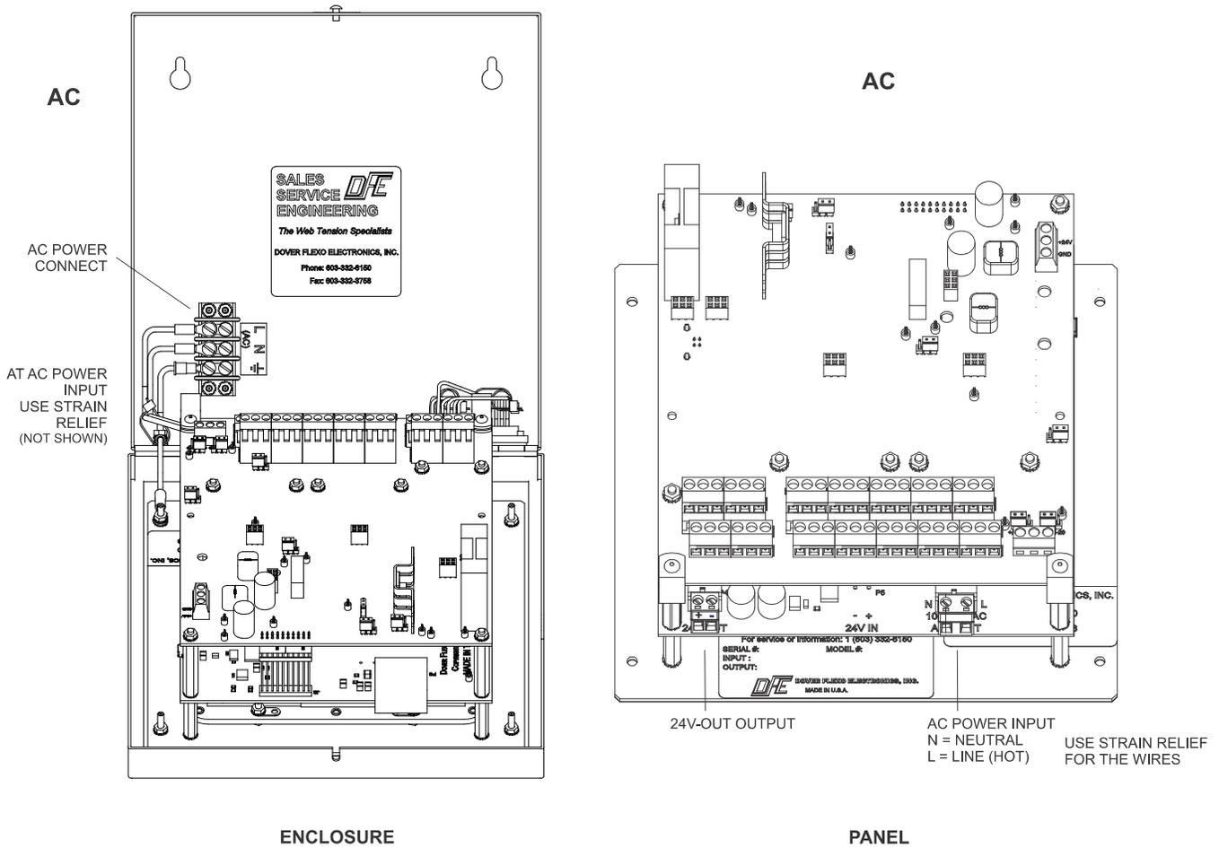
**Figure 11 – AC POWER ELECTRICAL CONNECTIONS**
