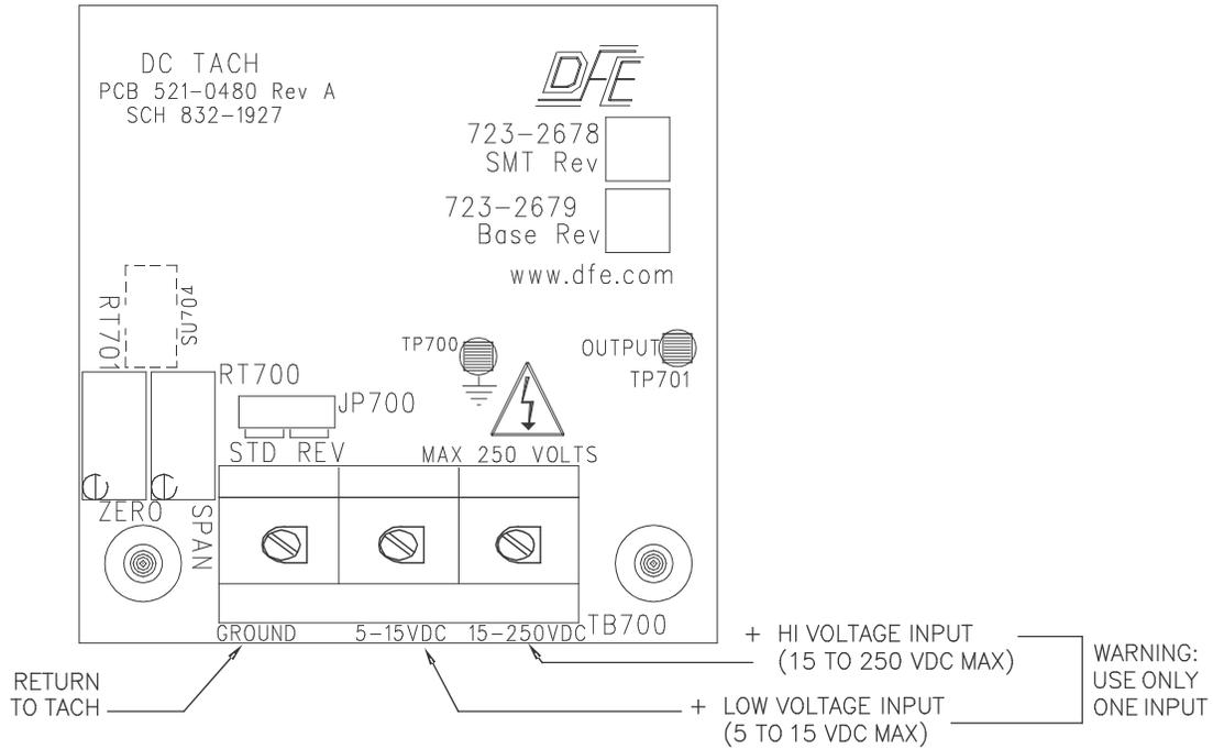
**Figure 16 – DC TACHOMETER ELECTRICAL CONNECTIONS**
