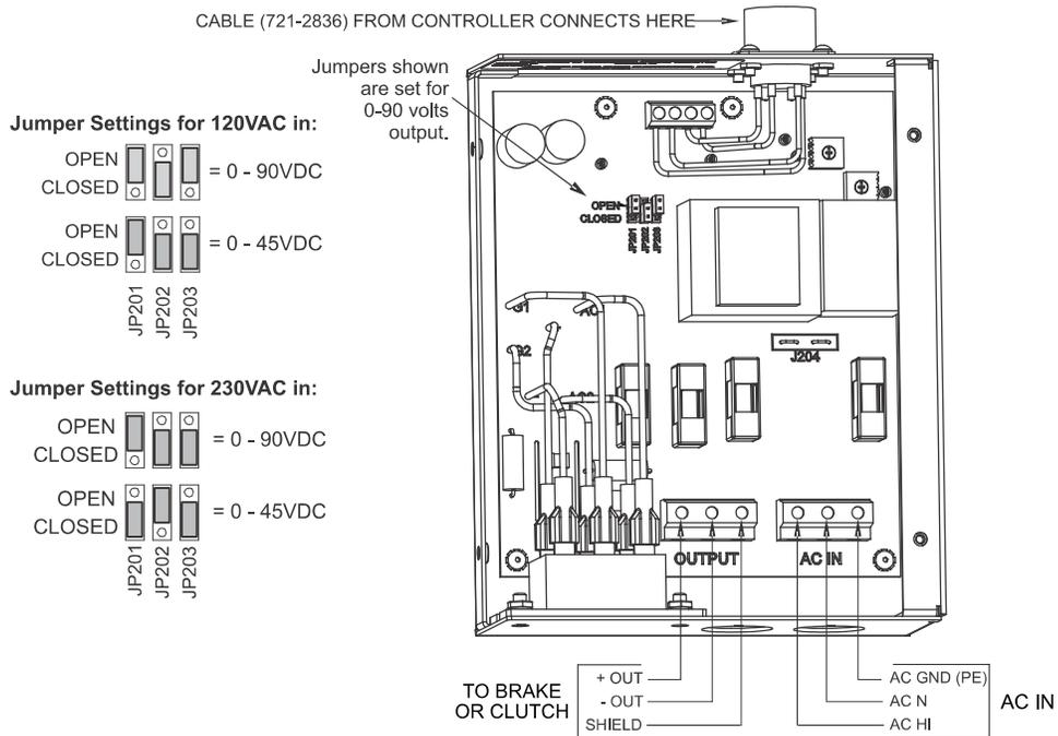
Figure 20 – HIGH VOLTAGE OUTPUT MODULE ELECTRICAL CONNECTIONS
