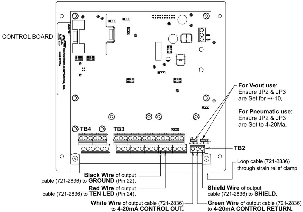
Figure 19 – EXTERNAL OUTPUT MODULE CABLE CONNECTIONS
