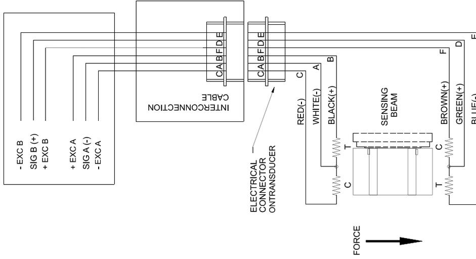
Figure 49 - MODELS RFA, LT, & VNW TRANSDUCER WIRING
