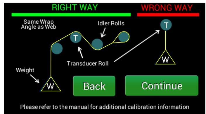
Figure 32 - WEB PATH FOR CALIBRATION
