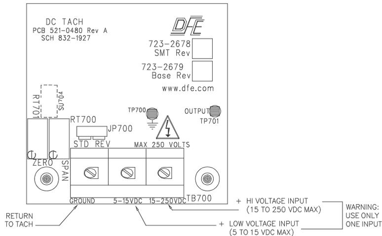
**Figure 36 - DC TACHOMETER CARD**
