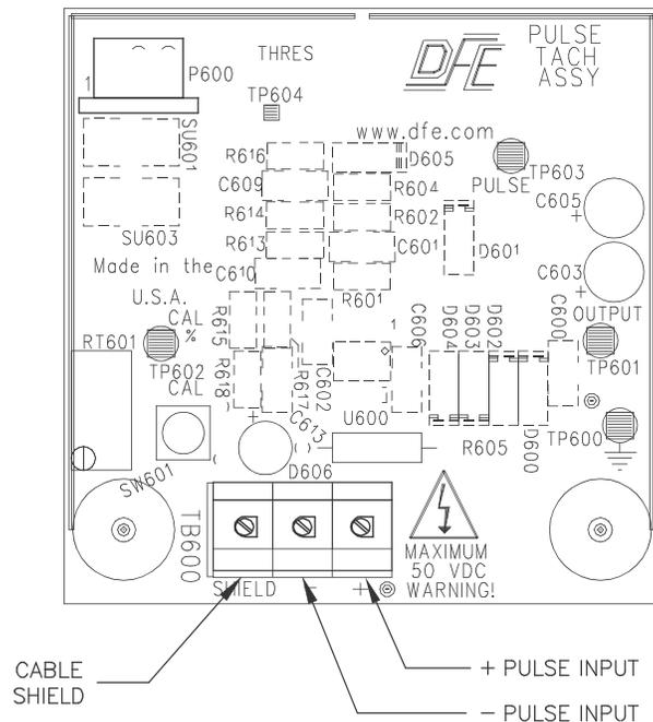
Figure 15 – PULSE TACHOMETER ELECTRICAL CONNECTIONS
