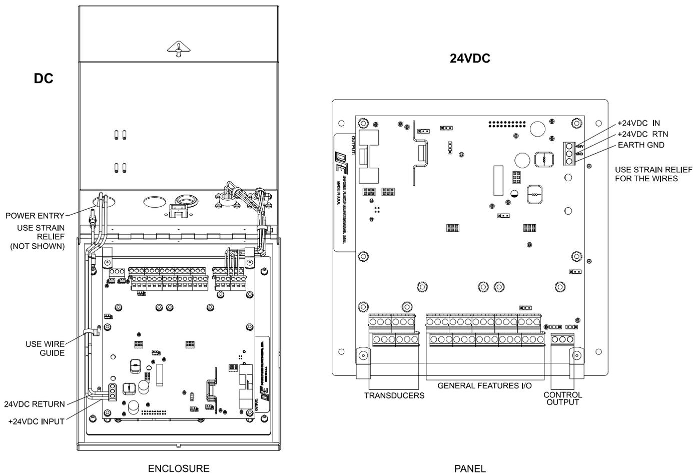
**Figure 10 – 24VDC POWER ELECTRICAL CONNECTIONS**
