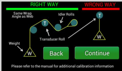
Figure 11 - WEB PATH FOR CALIBRATION
