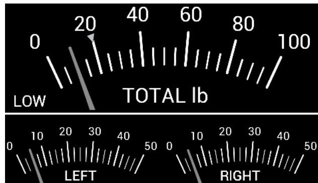
Figure 14 - TLS LOW ALARM SCREEN
