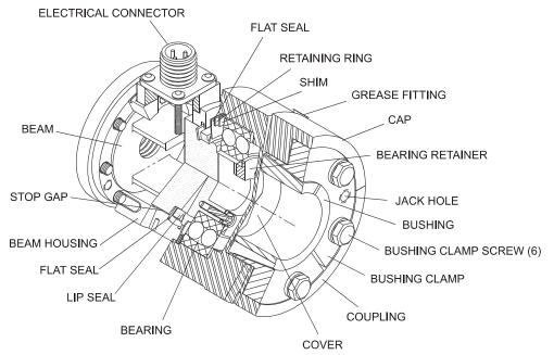
Figure 1 - LIVE SHAFT VERSION CUT-AWAY VIEW
