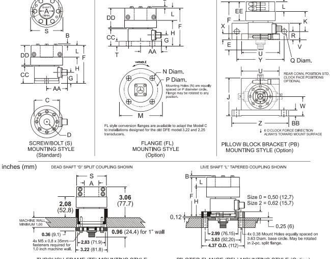
THROUGH-FRAME (TF) MOUNTING STYLE (Option) Size 2 Only PILOTED FLANGE (PFL) MOUNTING STYLE (Option) SIZE 0 & 2 ONLY (Replaces industry standard RFC style bearings)
