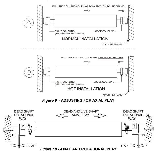
If no movement can be detected, loosen one shaft coupling and repeat the installation procedures, Section 2.4.3, A or B.
