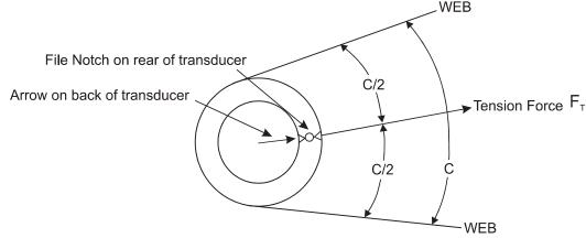
Figure 8 - TENSION FORCE DIRECTION
