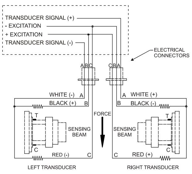
Figure 16 - MODEL C TRANSDUCER WIRING
