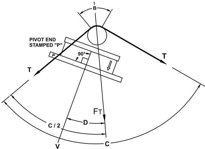
$$\text{TENSION NET FORCE} = \frac{(+)[4T\sin(B/2)][L\cos(D) + H\sin(D)]}{2L}$$
