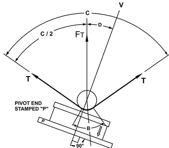
$$\text{TENSION NET FORCE} = \frac{(-)[4T\sin(B/2)][L\cos(D) + H\sin(D)]}{2L}$$
