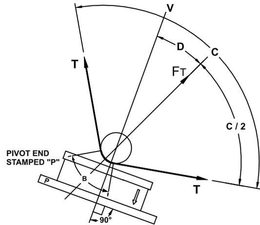
$$\text{TENSION NET FORCE} = \frac{(-)[4T\sin(B/2)][L\cos(D) - H\sin(D)]}{2L}$$
