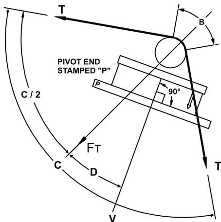
$$\text{TENSION NET FORCE} = \frac{(+)[4T\sin(B/2)][L\cos(D) - H\sin(D)]}{2L}$$
