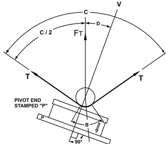
$$\text{TENSION NET FORCE} = \frac{(-)[4T\sin(B/2)][L\cos(D) + H\sin(D)]}{2L}$$
