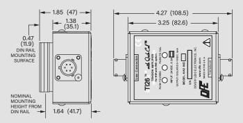
Shown with DIN Rail Clip option. Power input is 24 VDC.
