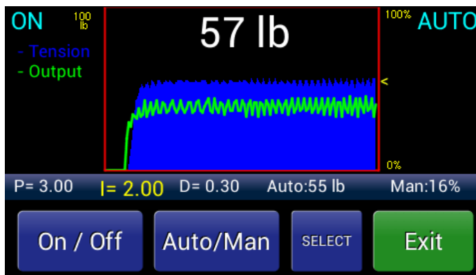
Figure 8-1 – TUNING SCREEN SHOWING OVERSHOOT
