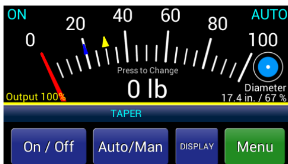
Figure 2-10 – TAPER SETPOINT ON METER
