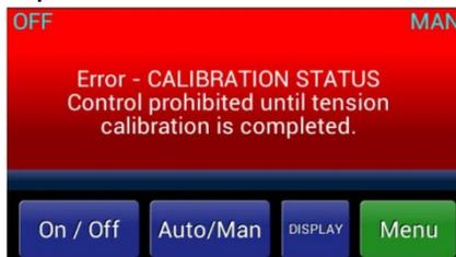
Before calibrating the unit, you should verify that the **Tension Units, Tension Range, Tension Source, Calibration Weight Percentage** and **Transducer Type** are set to values you desire. Press *Menu > Calibration Menu > Calibrate* buttons to get to the **Select Units** screen. Confirm that the preset units are correct, or choose your preferred units and then press **OK**.
