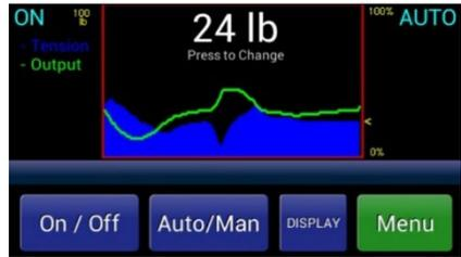
When in tension display screens, you may bring up velocity-sensitive “+” and “-” adjustment buttons by touching the tension display. These buttons, for adjusting the Auto Setpoint or Manual Output will time out a few seconds after discontinued use.
