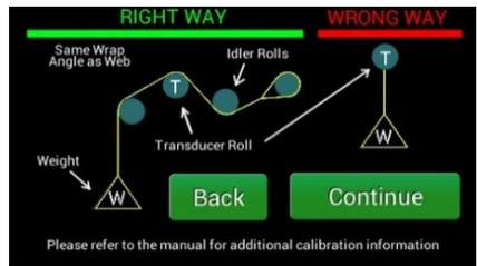
If additional calibration is required for inputs of Line Speed, Roll Speed or Roll Diameter, refer to **SECTION 6 - CALIBRATION of the The Manual**.
