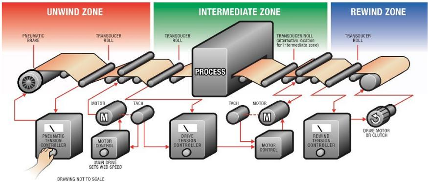
Some PID (Proportional, Integral and Derivative) tuning may be necessary to control tension optimally. Refer to **SECTION 6 - TUNING ADJUSTMENTS** of **The Manual** for a PID control overview and tuning procedure. Use the PID Tune View display located at *Menu > Calibration Menu > Tune PID Values* to adjust the PID terms for optimal control. See **SECTION 5 - USER INTERFACE OVERVIEW** of **The Manual** for information on how to utilize the **PID Tune View** display.
