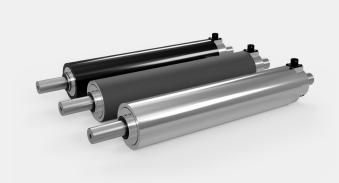
Ultimate performance and robust reliability set the Tension Roll® transducer apart from other sensing solutions on the market. A dead-shaft idler roller with tension sensors (load cells) integrated into each roll end, the Tension Roll® transducer is ideal for installation on original equipment or for retrofits since it arrives pre-assembled and ready-to-install between the facing sides of a machine frame.
