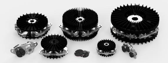
DFE brakes are designed for hassle-free operation, enabling friction pad changes in seconds, without tools. Cylinders can be actuated individually. Piston return springs prevent diaphragm puncture, increasing brake reliability and longevity.
