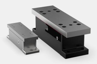
Model F Series transducers mount under pillow-block bearings at each end of an idler roll shaft. Designed for use in demanding tension measurement environments, the F transducer shell has a one-piece aluminum base with a removable stainless steel top plate. A rubber seal between the base and top plate prevents water ingress and dust contamination. The transducer's electrical connector is located at the end of a pig-tail cable for simpler access during installation.
