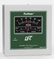
In addition to displaying average tension across the width of a running web, the TriView™ indicator also reads independent tension on both edges of a web process. This multi-zone monitoring allows the TriView™ to alert machine operators if manual adjustments are needed to equalize side-to-side tension and maintain optimum quality. Minimum and maximum tension limits can also be set to warn operators of potential web breaks, stretching or wrap-up incidents.
