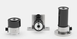
Patterned after the legendary Model C transducer, the RFA Ribbon Filament tension transducer's cantilevered form factor is ideal for wire, plastic, rubber, metal, glass, composite and other flexible substrates. Three standard wheels are available – ribbon (1"-4" wide), filament and an adapter wheel which functions as a hub for mounting custom wheels. Three mounting styles are available: Screw, Flange, and Pillow-Block.
