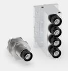
Compact, durable transducers for measuring light tension in fiber, filament or ribbon winding applications. The dual cantilevered beam provides torsional stiffness, strength and accuracy. Available in stackable or threaded through-frame mounting designs.
