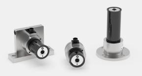
The VNW transducer measures process tension in narrow webs (up to four inches wide), ribbon or filament. It mounts cantilevered on process machinery for unwind/payoff, rewind/take-up or intermediate zone applications. Robust construction and impressive overload capability.
