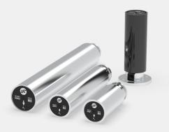
The NW transducer combines a cantilevered idler roll and two tension transducers in one integral unit — for fast, easy installation, high accuracy and web tracking performance. Roll widths from 6 to 20 inches (152 - 508 mm). Choose single-bolt mounting or a four-bolt flange.
