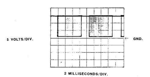
Turn the auto set pot. fully CCW. The pulse width of the waveform should gradually decrease as the firing circuit turns off. When fully off, the waveform at TP32 will be a straight line, 15 VDC above ground.
