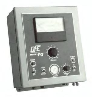
The P3 is very easy to operate. Simply turn the tension-setting knob until the meter displays the tension desired. The controller will automatically vary output air pressure to maintain correct tension regardless of changes in speed, roll diameter or brake/clutch characteristics. A soft-start circuit prevents brake lockup when starting with a slack web. Sample/hold and multiply/divide circuits provide smooth operation during flying splices on either unwind or rewind.
