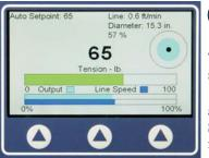
When in **Manual** mode, at the **Run** mode display, you can turn the rotary knob clockwise to increase your **Manual Tension Setpoint**. Turn the knob counter-clockwise to decrease the setpoint.
