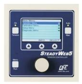
Before calibrating the unit, you should verify that the **Tension Units** and the **Tension Range** are set to the values you prefer. Press the **Menu/Run** button to access the Main Menu screen.
