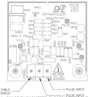
Figure 15 – PULSE TACHOMETER ELECTRICAL CONNECTIONS
