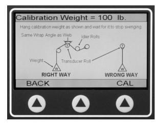
Figure 30 - WEB PATH FOR CALIBRATION
