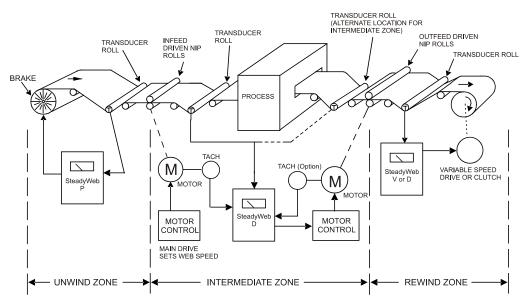
Figure 2 - EXAMPLES OF TENSION ZONES
