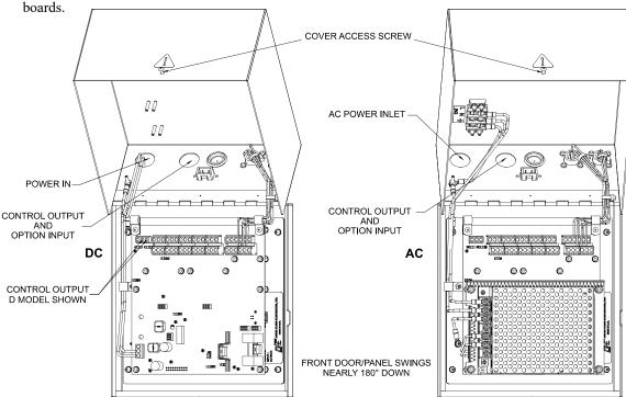
Figure 7 - ENCLOSURE VERSION SERVICE ACCESS
