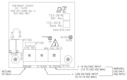
Figure 32 - DC TACHOMETER CARD
