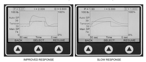
Figure 36 - TUNING SCREENS SHOWING ADJUSTMENT RESPONSES
