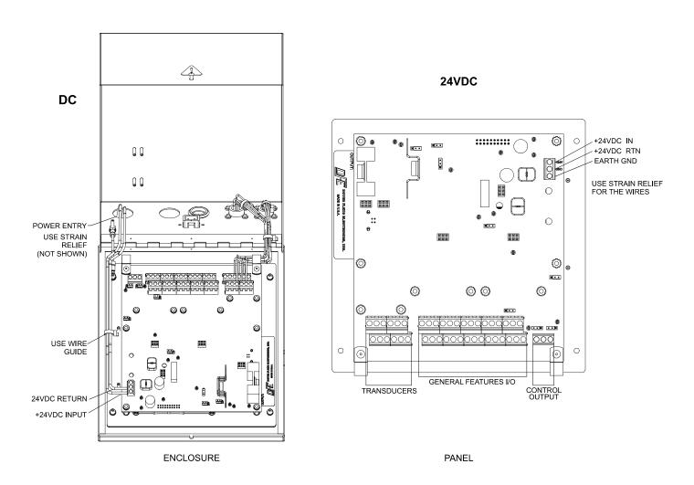
Figure 10 - 24VDC POWER ELECTRICAL CONNECTIONS
