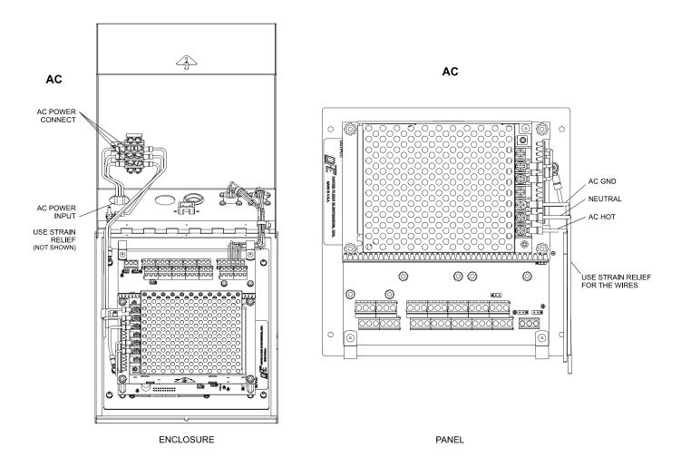
Figure 11 – AC POWER ELECTRICAL CONNECTIONS
