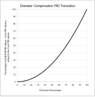
Figure 39 - DIAMETER COMPENSATION PID TRANSITION
