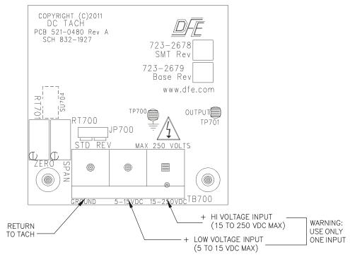
Figure 16 - DC TACHOMETER ELECTRICAL CONNECTIONS
