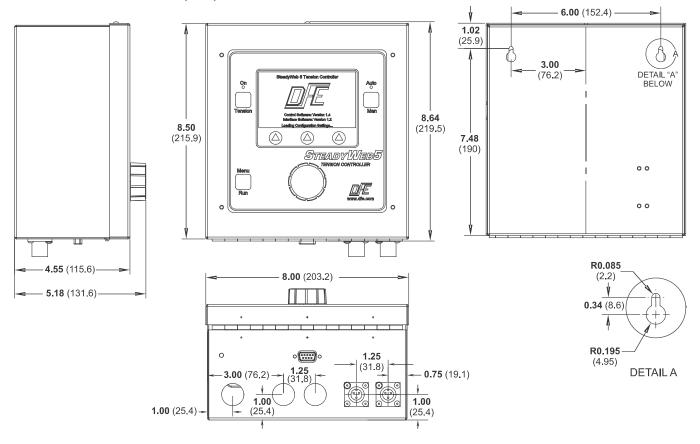
Figure 3 - ENCLOSURE VERSION DIMENSIONS and VIEWS
