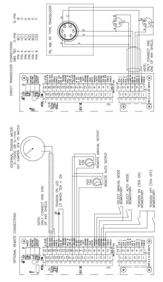
Figure 13 - CONTROL BOARD TRANSDUCER ELECTRICAL CONNECTIONS AND REMOTE OPTION
