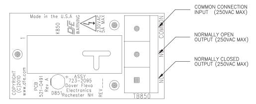
Figure 17 - RELAY ELECTRICAL CONNECTIONS
