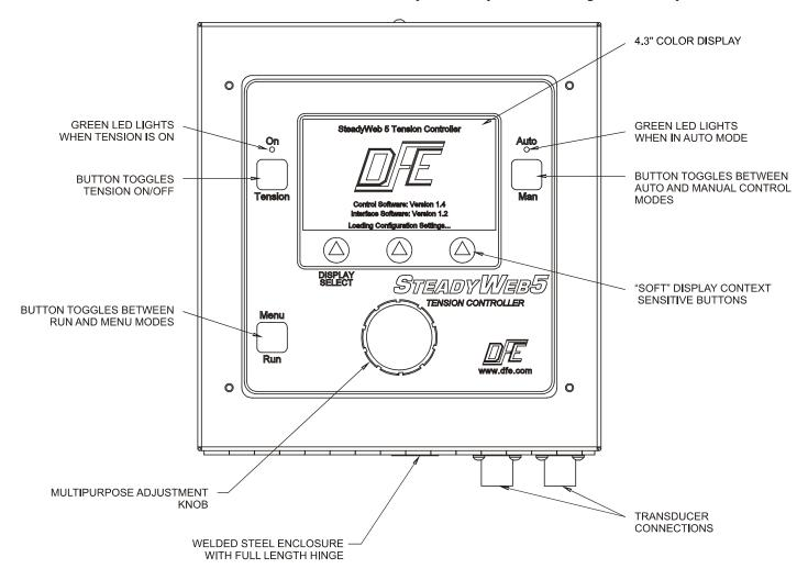
Figure 1 - FRONT VIEW OF STEADYWEB™5
