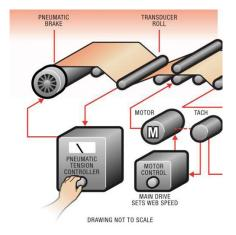
Then, as the web machine runs, tension on the transducer-equipped idler roller is measured and read by the controller. A special comparison circuit looks at both the set point and the actual measured web tension, the difference of which is an error signal. Because web processes are dynamic systems, tension in any zone tends to change from moment to moment, typically running less than or
