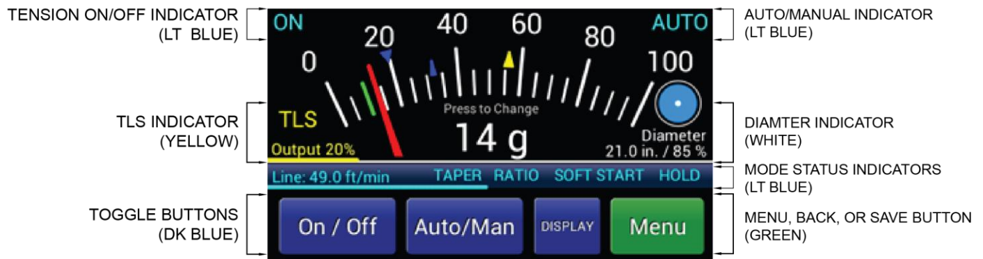
Figure 1-2 - LOCATIONS OF TOGGLE BUTTONS / INDICATORS IN DISPLAY
