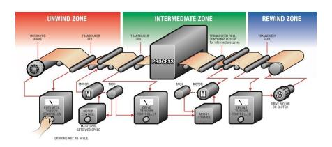
Some PID (Proportional, Integral and Derivative) tuning may be necessary to control tension optimally. Refer to **SECTION 6** - **TUNING ADJUSTMENTS** of **The Manual** for a PID control overview and tuning procedure. Use the PID Tune View display located at *Menu > Calibration Menu > Tune PID Values* to adjust the PID terms for optimal control. See **SECTION 5** - **USER INTERFACE OVERVIEW** of **The Manual** for information on how to utilize the **PID Tune View** display.
