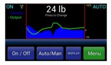
When in tension display screens, you may bring up velocitysensitive "+" and "-" adjustment buttons by touching the tension display. These buttons, for adjusting the Auto Setpoint or Manual Output will time out a few seconds after discontinued use.
