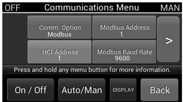
Figure 7 - SETUP MODBUS COMM
