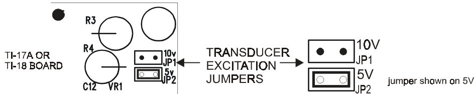
Figure 6 - TRANSDUCER VOLTAGE JUMPERS
