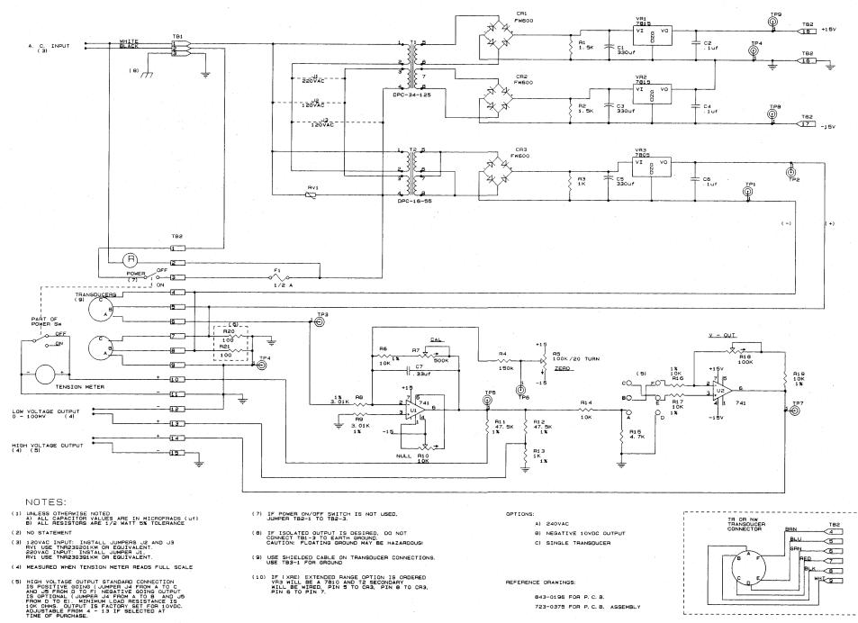
(6) R20 AND R21 ARE INSTALLED WHEN A SINGLE TRANSDUCER IS USED WITH A PANEL ONLY INDICATOR. CONNECT THE TRANSDUCER TO TB2-4, 5, 6.
