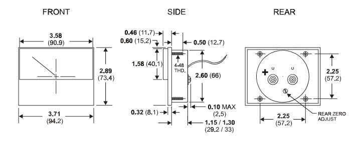
Figure 4 - REMOTE TENSION METER (Accessory)
