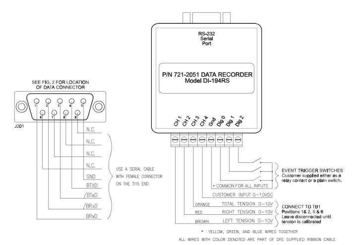
Figure 35 - COMPUTER INTERFACE (CI) DATA RECORDER CONNECTIONS
