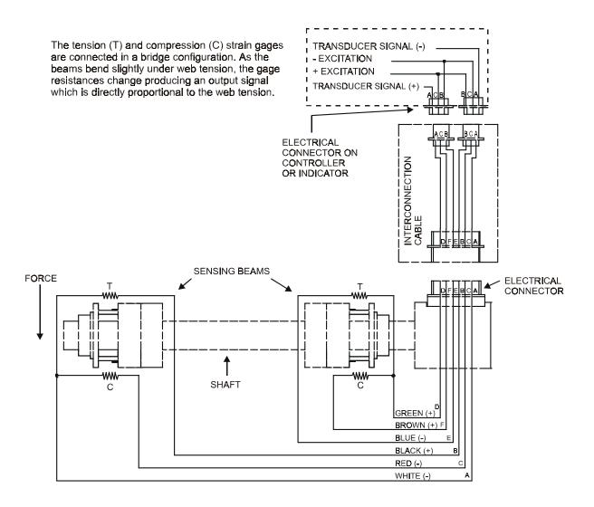
Figure 42 - TR & NWI TRANSDUCER WIRING
