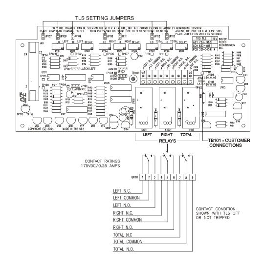
Figure 36 - TENSION LIMIT SWITCH RELAY CONNECTIONS
