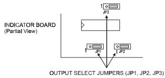
Figure 19 - DIFFERENTIAL OUTPUT JUMPERS
