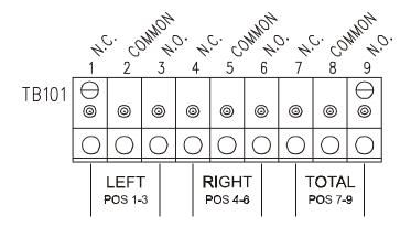
Figure 24 - TENSION LIMIT SWITCH CONNECTIONS
