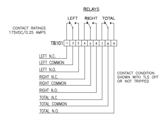
Figure 9 - TENSION LIMIT SWITCH (TLS) OPTION RELAY CONTACTS
