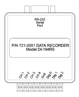
Figure 33 - COMPUTER INTERFACE (CI) DATA RECORDER MODULE
