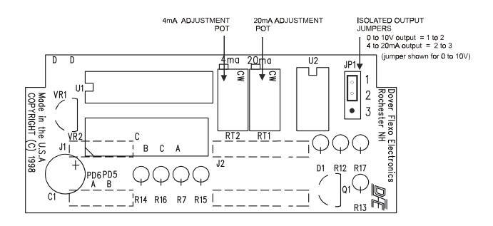
Figure 31 - ISOLATED OUTPUT BOARD
