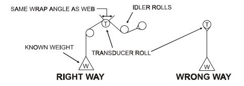
Figure 10 - WEB PATH FOR METER CALIBRATION
