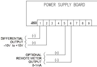
Figure 20 - DIFFERENTIAL OUTPUT CONNECTION and OPTIONAL REMOTE METER
