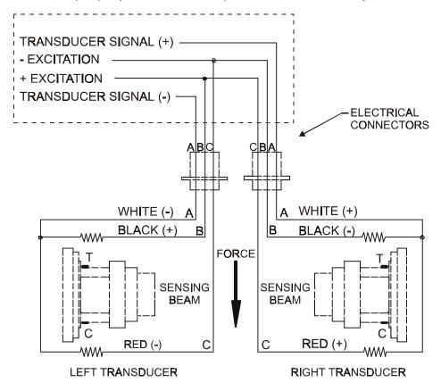
Figure 41 - MODELS C, RS, & UPB TRANSDUCER WIRING
