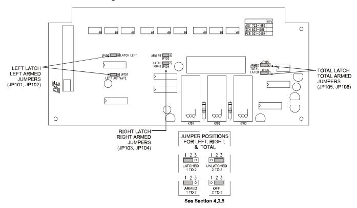
Figure 38 - TENSION LIMIT SWITCH BOARD JUMPERS
