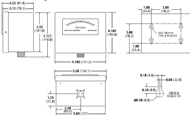
Figure 6 - REMOTE METER ENCLOSURE DIMENSIONS
