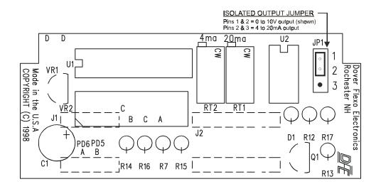
Figure 39 - ISOLATED OUTPUT BOARD JUMPERS (See Section 4.3.4)
