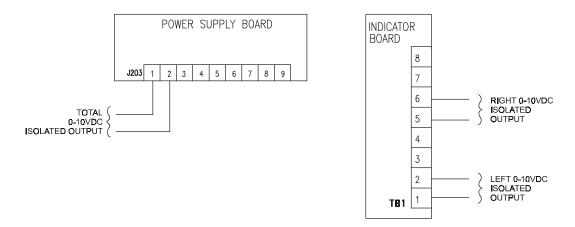
Figure 22 - ISOLATED OUTPUT CONNECTIONS
