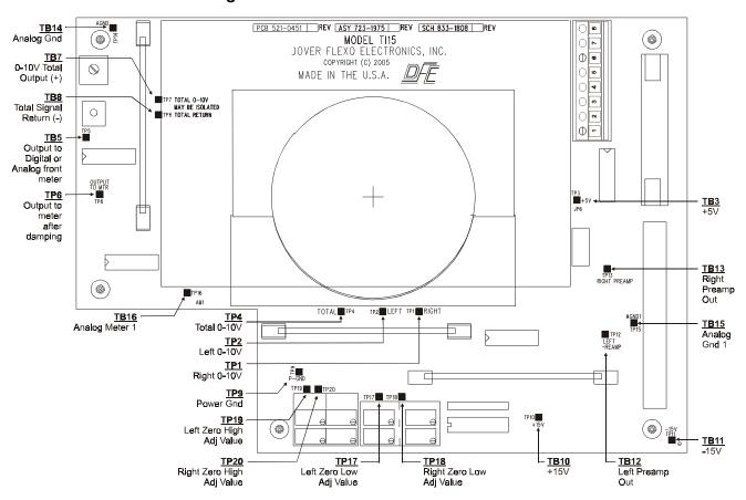
Figure 26 - INDICATOR TEST POINTS
