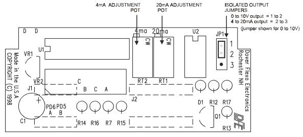
Figure 21 - ISOLATED OUTPUT JUMPERS and ADJUSTMENTS
