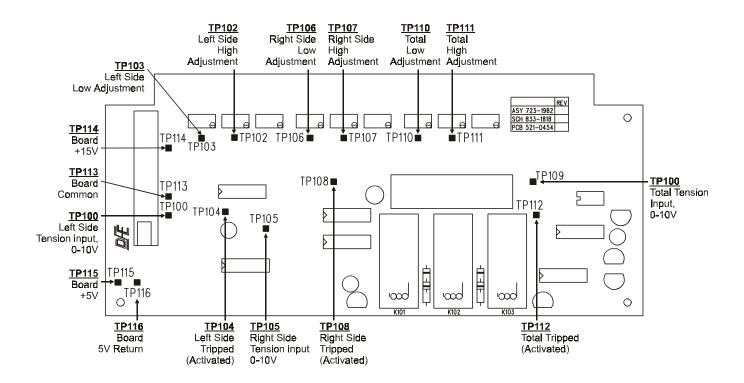
Figure 27 - TENSION LIMIT SWITCH BOARD TEST POINTS
