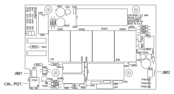
Figure 18 - DIGITAL METER BOARD
