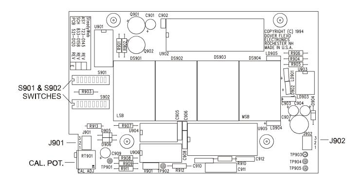
Figure 32 - DIGITAL METER BOARD
