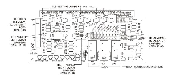
Figure 30 -TENSION LIMIT SWITCH BOARD
