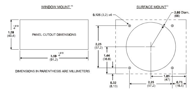
Figure 5 - REMOTE METER MOUNTING DIMENSIONS
