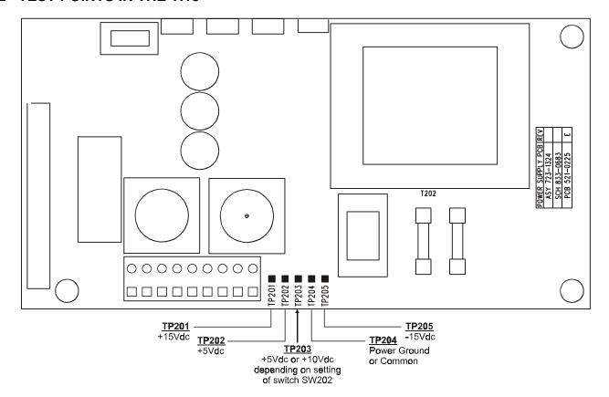
Figure 25 - POWER BOARD TEST POINTS
