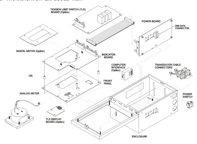
Figure 2 - TI15 INDICATOR - EXPLODED VIEW
