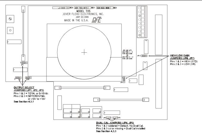
Figure 37 - INDICATOR BOARD JUMPERS
