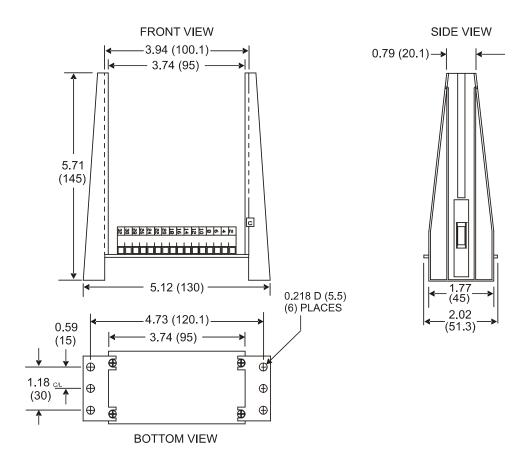
Figure 3 - ACCESSORY PLUG-IN CARD ADAPTER DIMENSIONS
