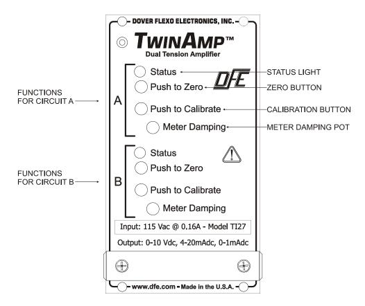
Figure 1 - FRONT VIEW OF TWINAMP™
