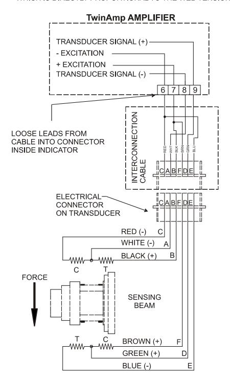
Figure 15 - RFA TRANSDUCER WIRING
