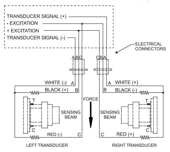
Figure 14 - MODELS C, RS, & F TRANSDUCER WIRING
