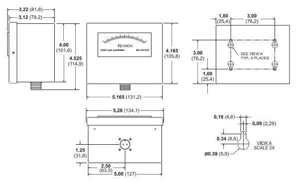
Figure 5 - ACCESSORY TENSION METER ENCLOSURE DIMENSIONS
