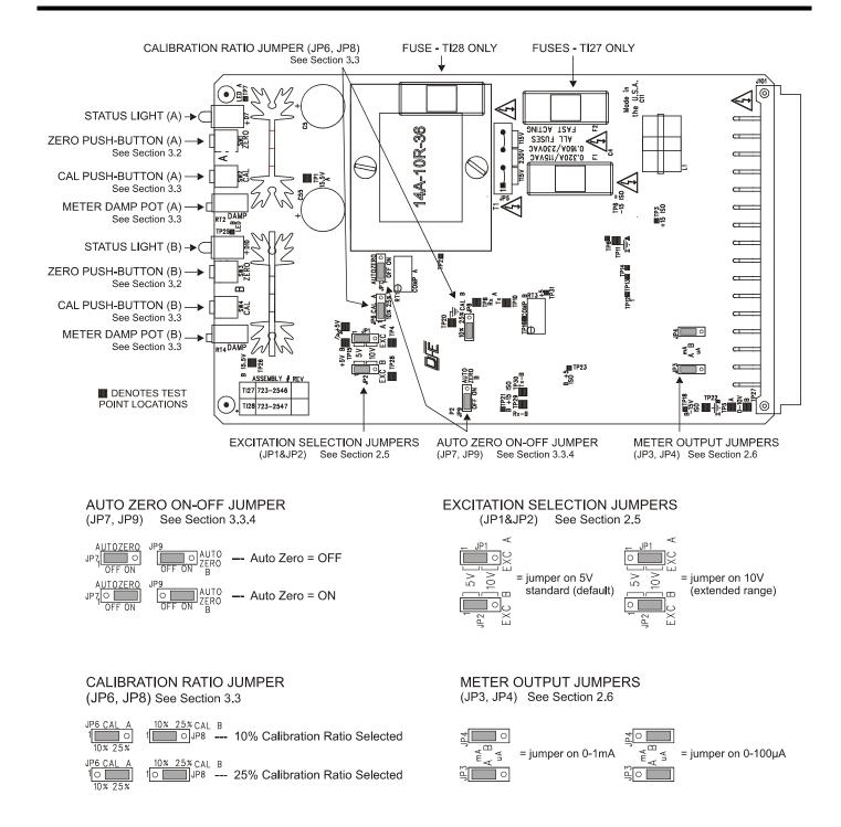
Figure 12 - TWINAMP PC BOARD SHOWING COMPONENT LOCATIONS (Simplified for clarity)0
