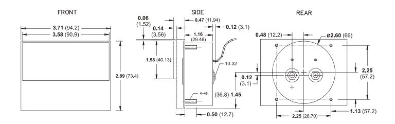
Figure 4 - ACCESSORY TENSION METER DIMENSIONS
