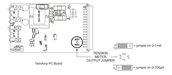
Figure 7 - TENSION METER OUTPUT JUMPERS
