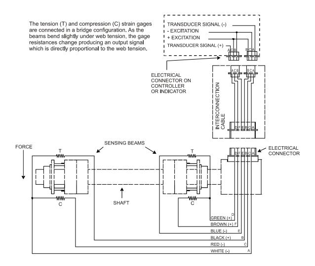
Figure 16 - TR & NW TRANSDUCER WIRING
