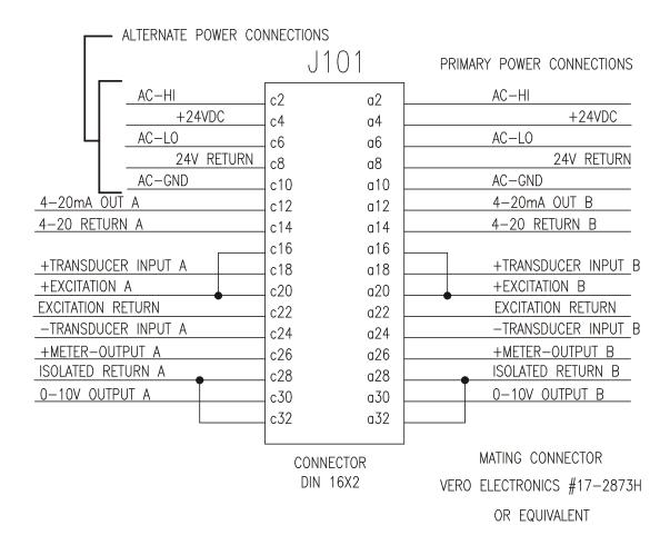
Figure 8 - STANDARD ELECTRICAL CONNECTIONS
