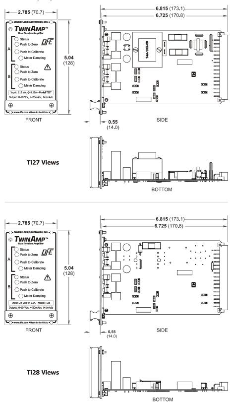
Figure 2 - Ti27 and Ti28 UNIT DIMENSIONS and VIEWS
