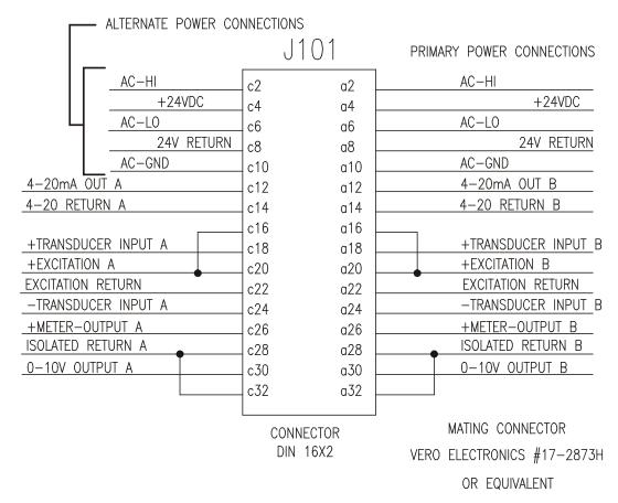
Figure 13 - STANDARD ELECTRICAL CONNECTIONS
