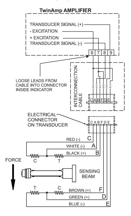
Note: Extended Range Option (XR) must be used with LT Transducers
