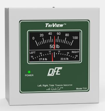
The TriView™ LRT tension indicator works with a Tension Roll® transducer or a transducer pair (mounted on each end of an idler roll) to independently measure both sides of web tension.
