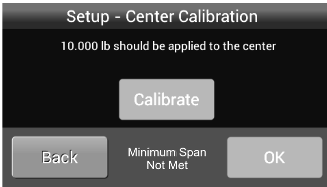
Figure 25 - CENTER CALIBRATION NOT READY
