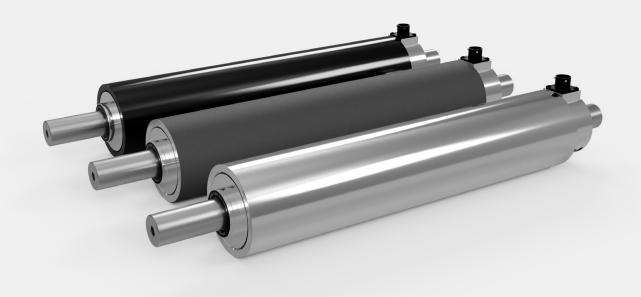
Ultimate performance and robust reliability set the Tension Roll® Transducer apart from other web sensing solutions on the market. A dead-shaft idler roller with tension sensors (load cells) integrated into each roll end, the Tension Roll® is ideal for installation on original equipment or for retrofits since it arrives pre-assembled and ready-to-install between the facing sides of a machine frame.
