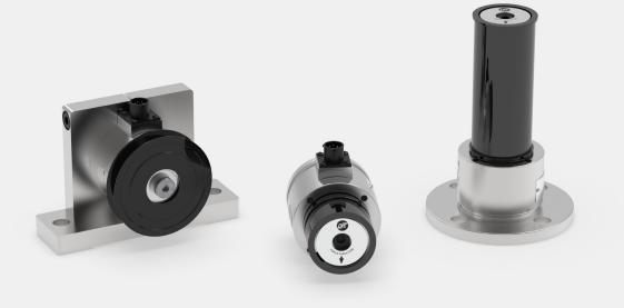
The VNW (Very Narrow Web) transducer combines the robustness of DFE's Model C transducer with the choice of mounting styles and wheel options from the cantilevered RFA load cell design. Typical applications include wire, plastic, rubber, metal, glass and other flexible substrates. The VNW's maximum 400 lb load rating extends it's measurement capability beyond the RFA's limit of 150 lbs, allowing for higher tension applications such as steel belt and tire cord.
