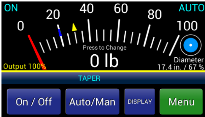
Figure 16 - TAPER SETPOINT ON METER
