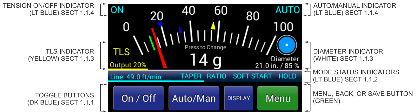
Figure 2 – LOCATIONS OF TOGGLE BUTTONS / INDICATORS IN DISPLAY
