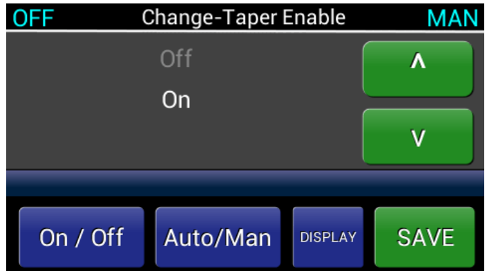
Figure 14 - ENABLE TAPER TENSION
